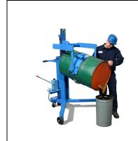
82 – Drum palletizer with manual lift and hand crank tilt
