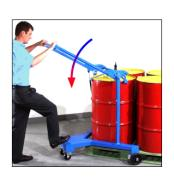
**81 Drum Spotter –** Used to move rimmed drums on to and off of pallets
